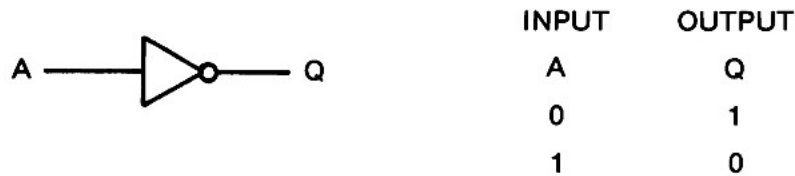
Figure 2.1 Inverter Diagram and Truth Table.
