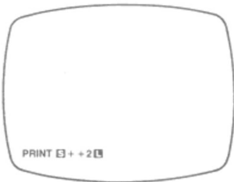
The [ ] is the *syntax error marker* (the syntax is the grammar of messages, saying which are allowed and which are not); it shows that the computer got as far as "PRINT," but after that it was not a "legal" message.
