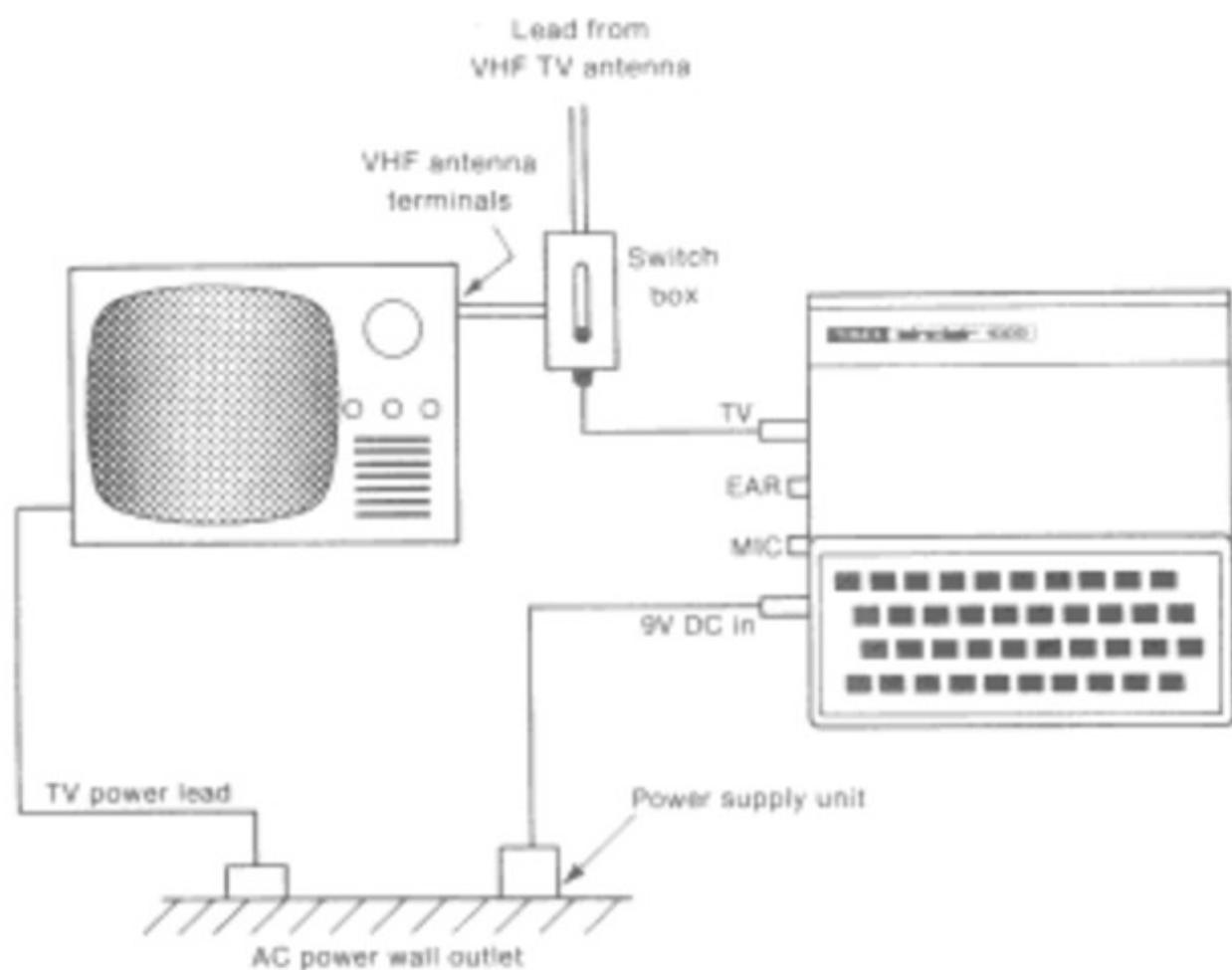
Second, plug the power supply into the wall and into the 9V DC IN socket on the computer.
