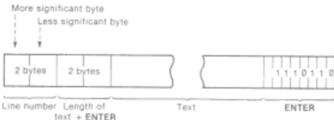
Note that, in contrast with all other cases of two-byte numbers in the Z80, the line number here (and also in a **FOR-NEXT** control variable) is stored with its more significant byte first: that is to say, in the order that you would write them down.
