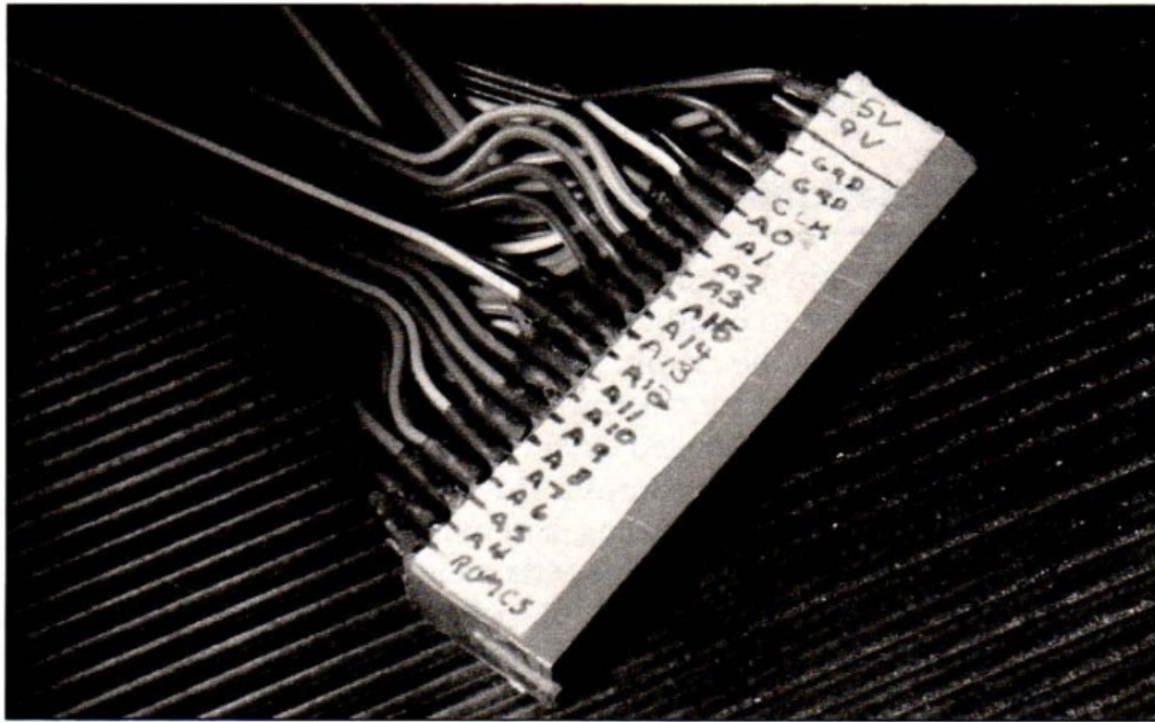
Figure 3.13 The completed backplane adapter.
