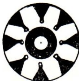
Figure 6.21 A diagram of the wiper assembly to transmit wind direction. The outer contacts connect to the data lines. The center track connects to ground.
