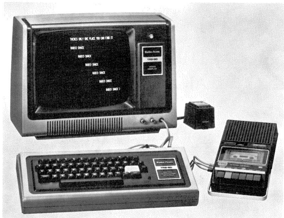
The TRS-80 personal computer distributed through Radio Shack stores. With this machine use the ENTER key instead of CARRIAGE RETURN. The Level II BASIC supplied with this machine is very similar to BASIC-PLUS.
