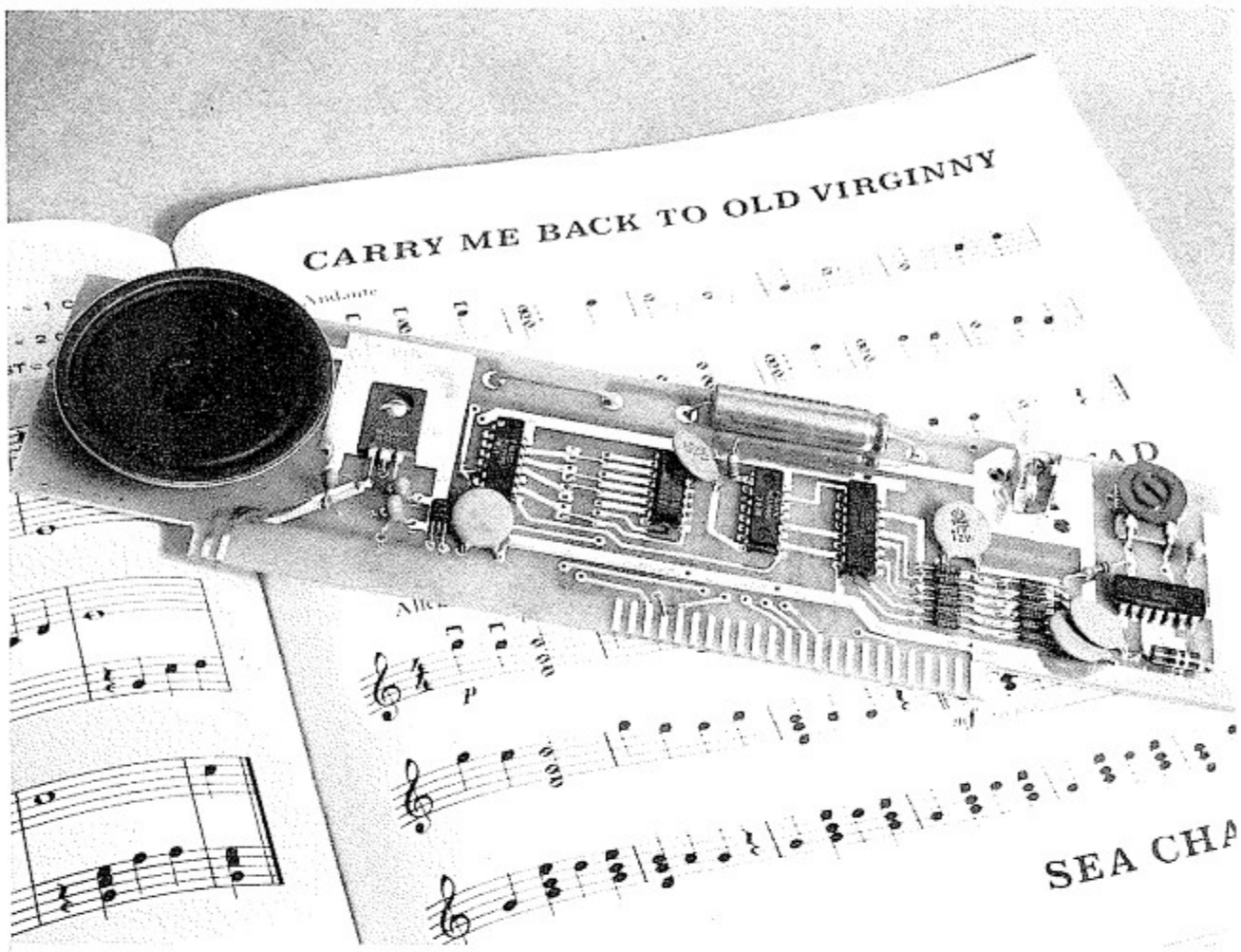
Fig. 14-2. A music synthesizer board for the S-100 bus. (Courtesy Newtech Computer Systems)
