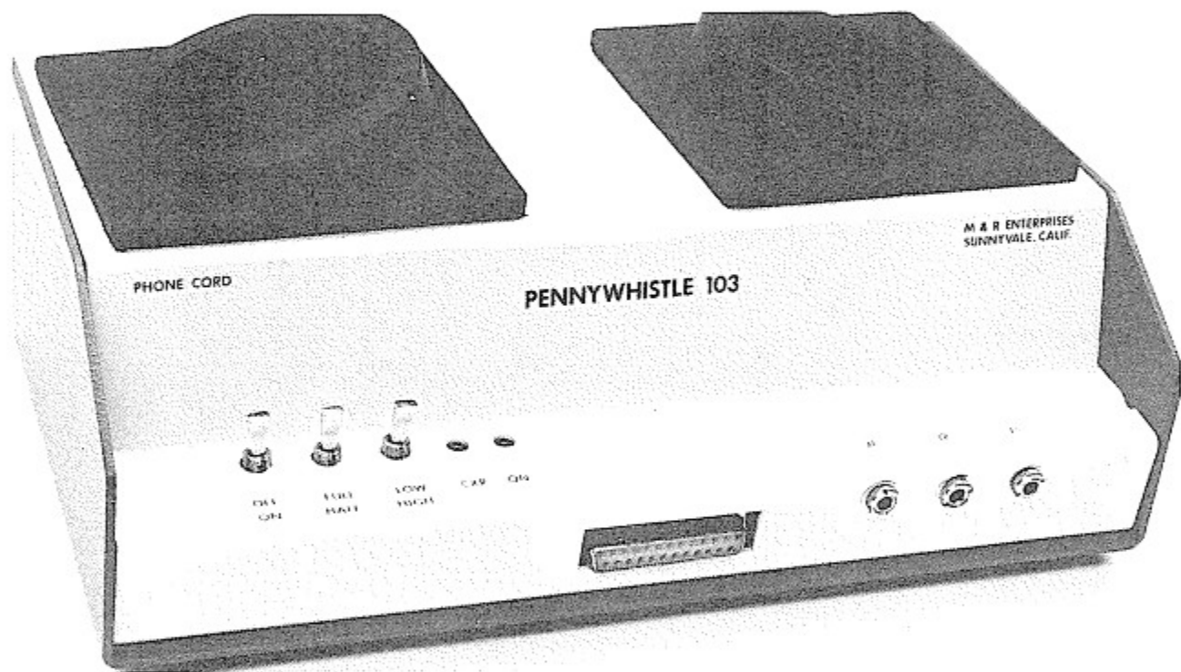
Fig. 7-20. A typical modem using an acoustical coupler.
