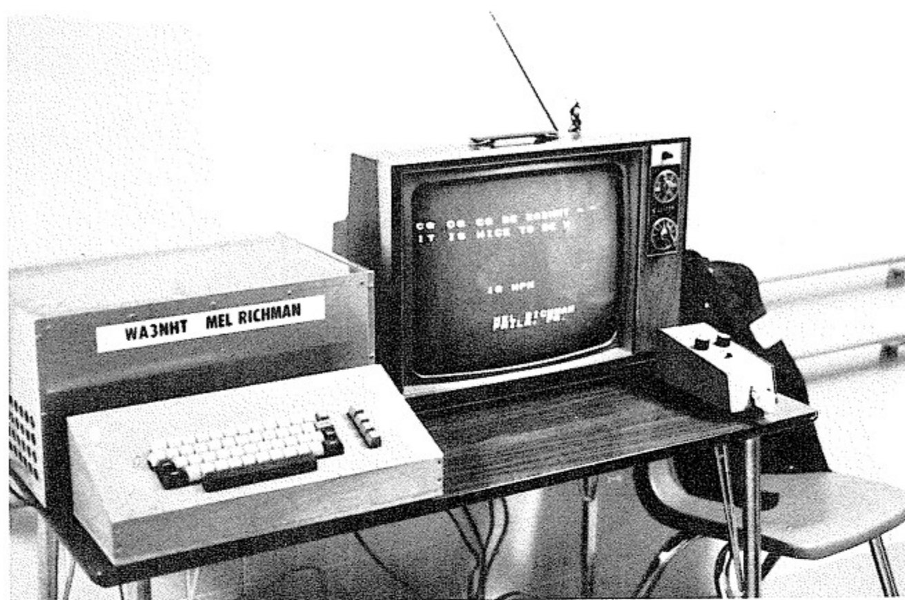
Fig. 14-3. Using a microcomputer to transmit and receive Morse code.
