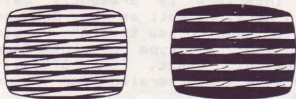
Left screen shows volume too low; right screen shows correct volume.
