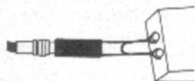
UHF/VHF matching transformer
