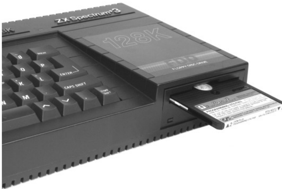
Fig 1.11 The 3 inch drive was located to the right of the keyboard. Disks had to be turned over in order to access all 360K storage capacity.
