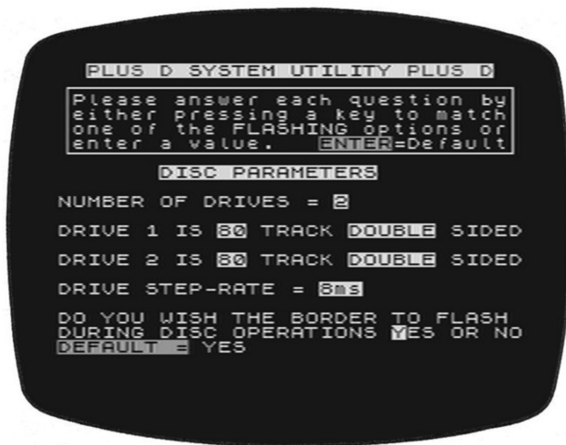
Fig 3.6 The Plus D System Tape running on Spectaculator. Just accept all the default values for your disk drive; answer no for the printer question that follows this screen, however, to avoid a lengthy printer questionnaire.
