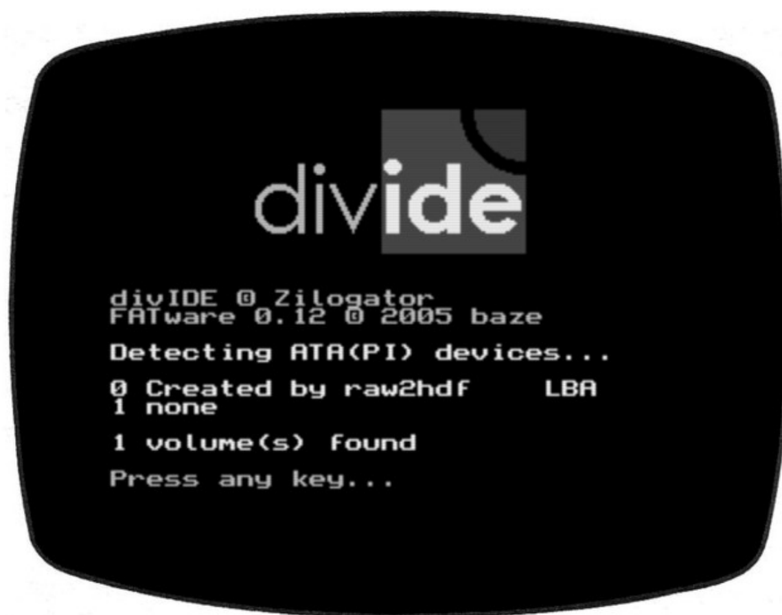
Fig 8.1 DivIDE boots, recognising a hard disk connected.
