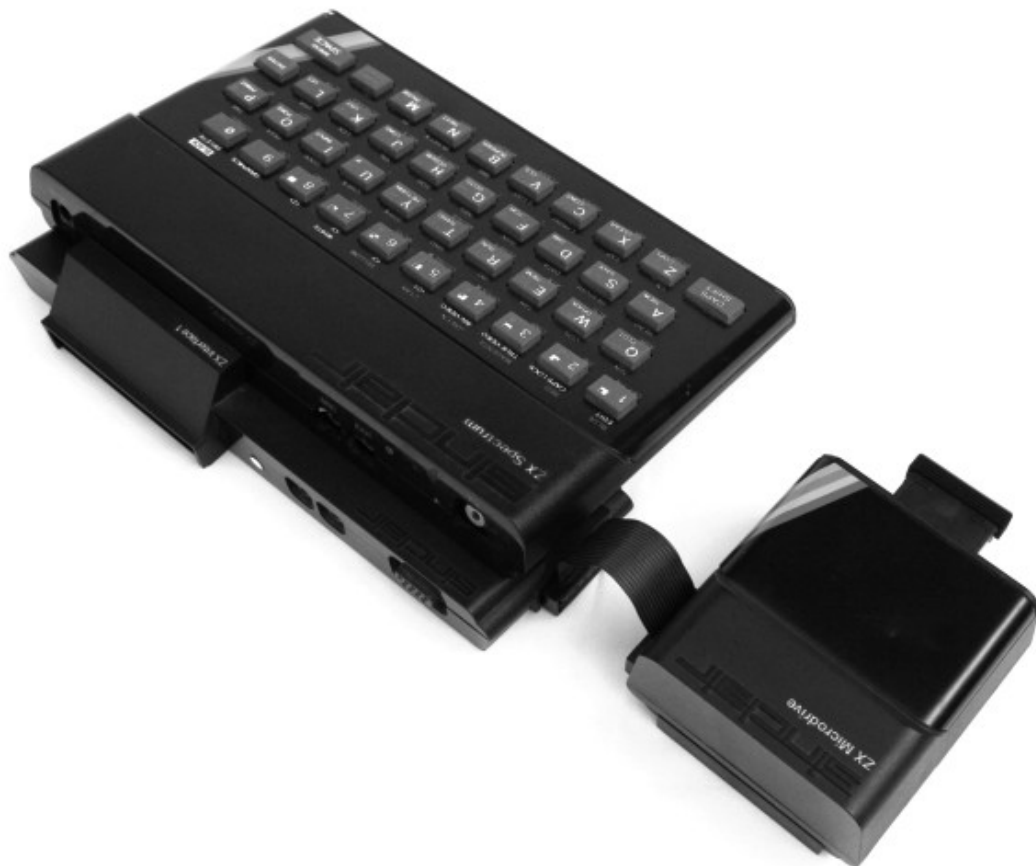
Fig 1.9 The Microdrive plugged into the Interface 1, which sat beneath the Spectrum. Up to eight in a row could be connected.
