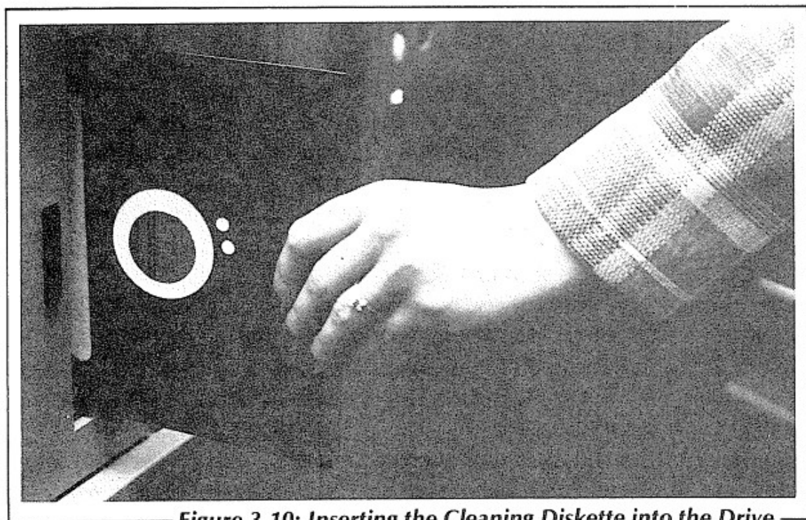
—Figure 3.10: Inserting the Cleaning Diskette into the Drive—
