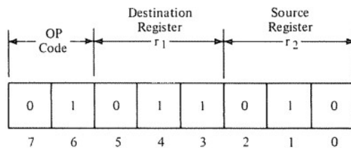
Figure 2-2 Instruction Format for Internal CPU Register Transfer
