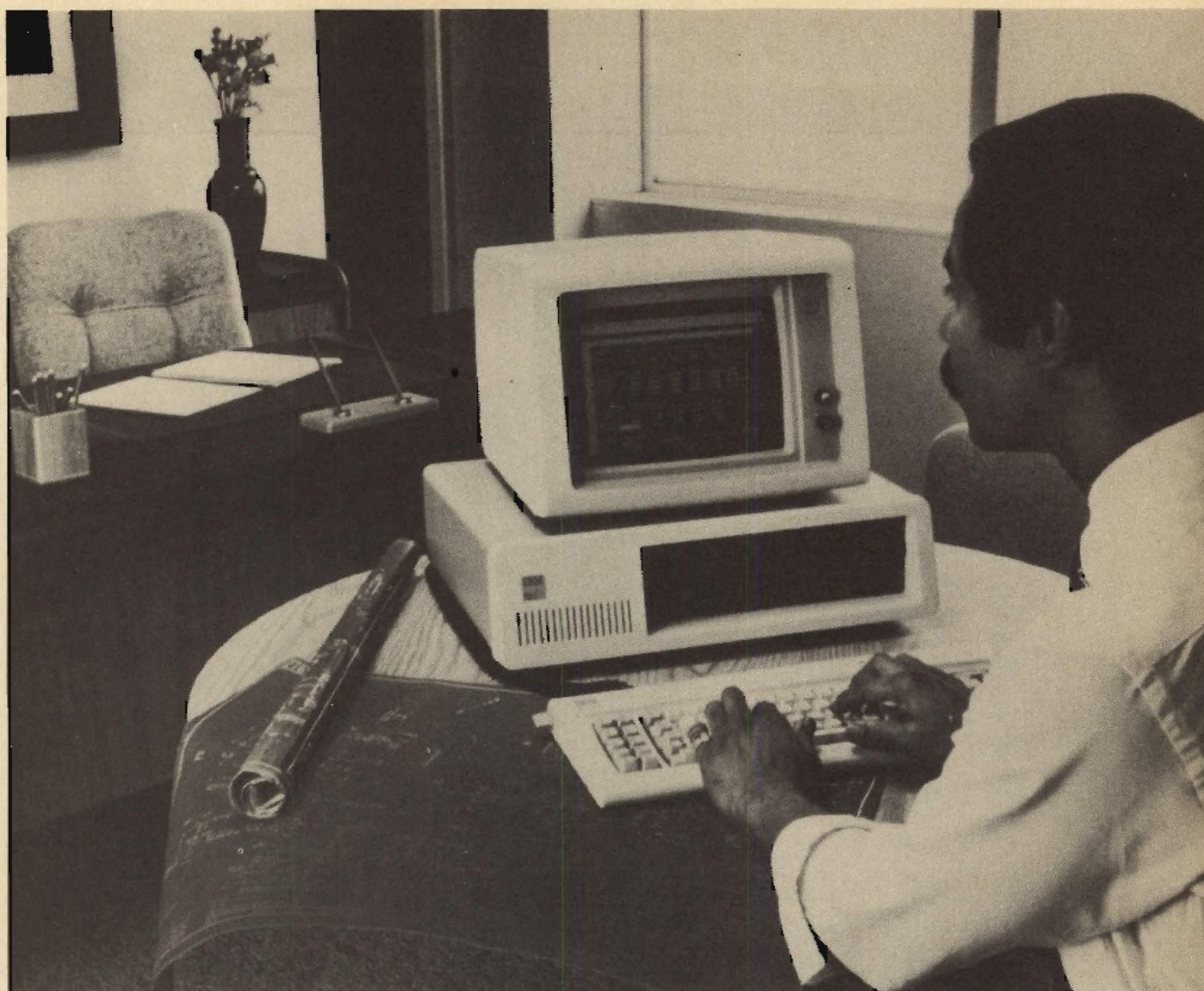
The typical home computer consists of a keyboard to type information in and a video screen to display it. The computer's brains may be in a separate box, or built into the keyboard or the display.
