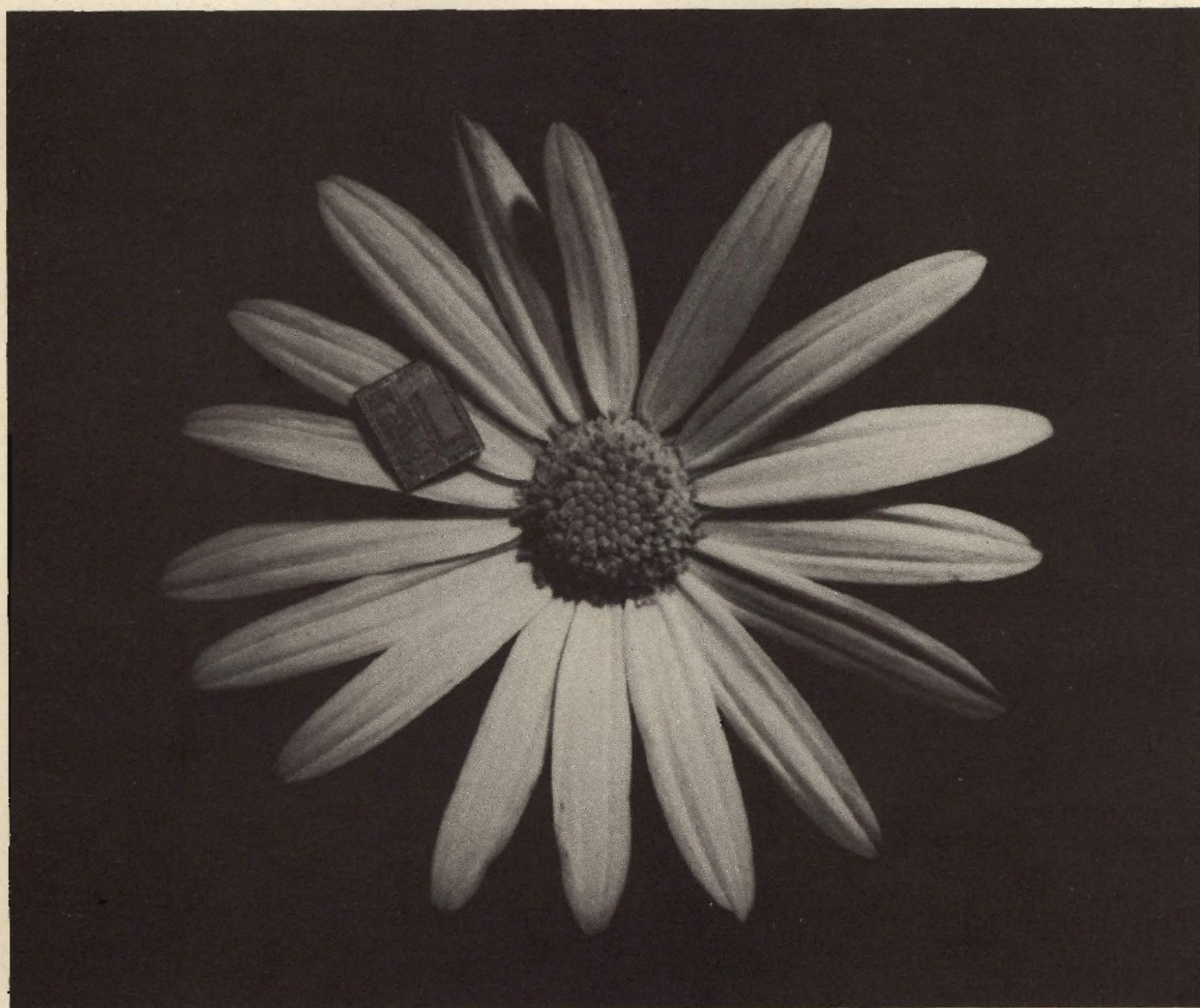
The microprocessor chip, so tiny it's dwarfed by a daisy, is the real brains of the computer. It's made of silicon, and etched with thousands of electronic circuits—the transistors that actually do the computing.
