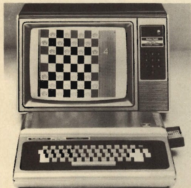
Radio Shack's TRS-80 Color Computer can display eight colors; a wide range of software is available.
