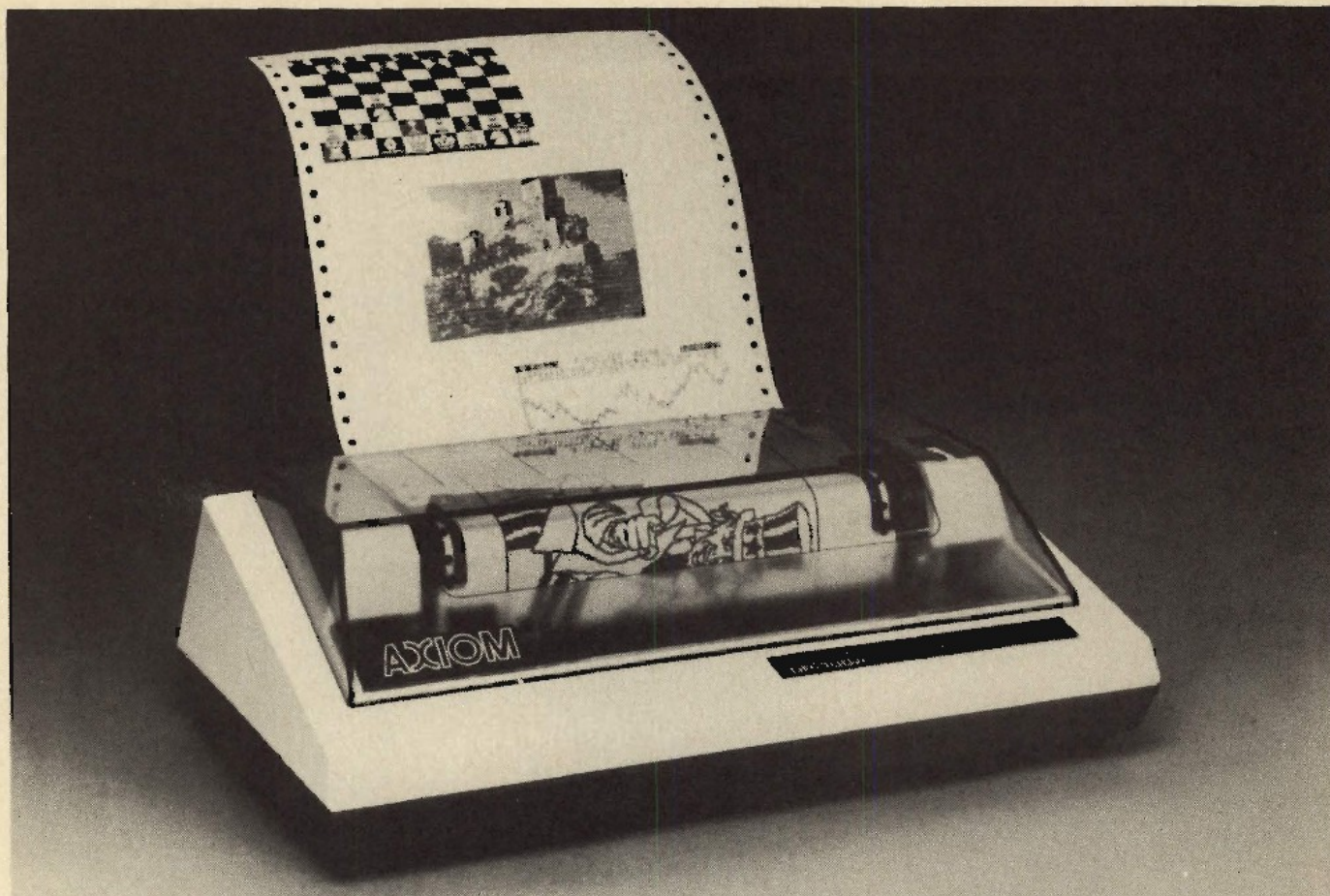
The most sophisticated dot-matrix printers can produce amazingly detailed images. If this capability is available, it's probably worth getting; it may not add significantly to the printer's price.
