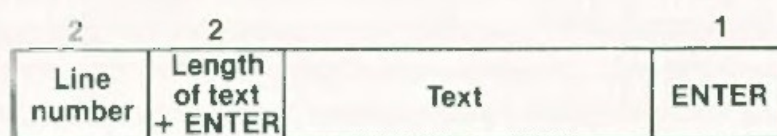
Fig. 4.2. Format of a BASIC line.
