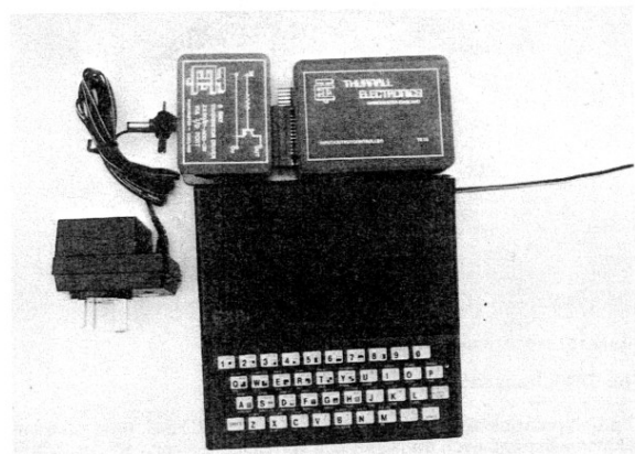
Figure 17a: ZX81, TE10 and TE15 and power supply, showing power supply inputs all connected
