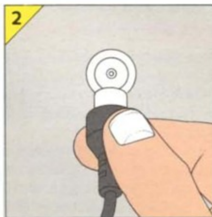
2 Detach the aerial cable from your television set. Insert the other plug on the Spectrum's aerial lead into the aerial socket.
