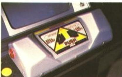
The snappy control unit which you use to tilt the screen. Flipper buttons are on the side.
