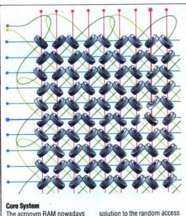
The acronym RAM nowadays always refers to electronic microchip devices, but for 20 years the ferro-magnetic core system illustrated here was the cheapest, fastest, most elegant solution to the random access memory problem. Binary data was represented by the magnetic polarity of the iron rings
