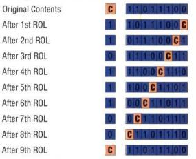
You can see from this demonstration that the original contents of the carry flag (C) do not particularly concern us, as this is rotated through the byte and eventually shifted out of the byte
