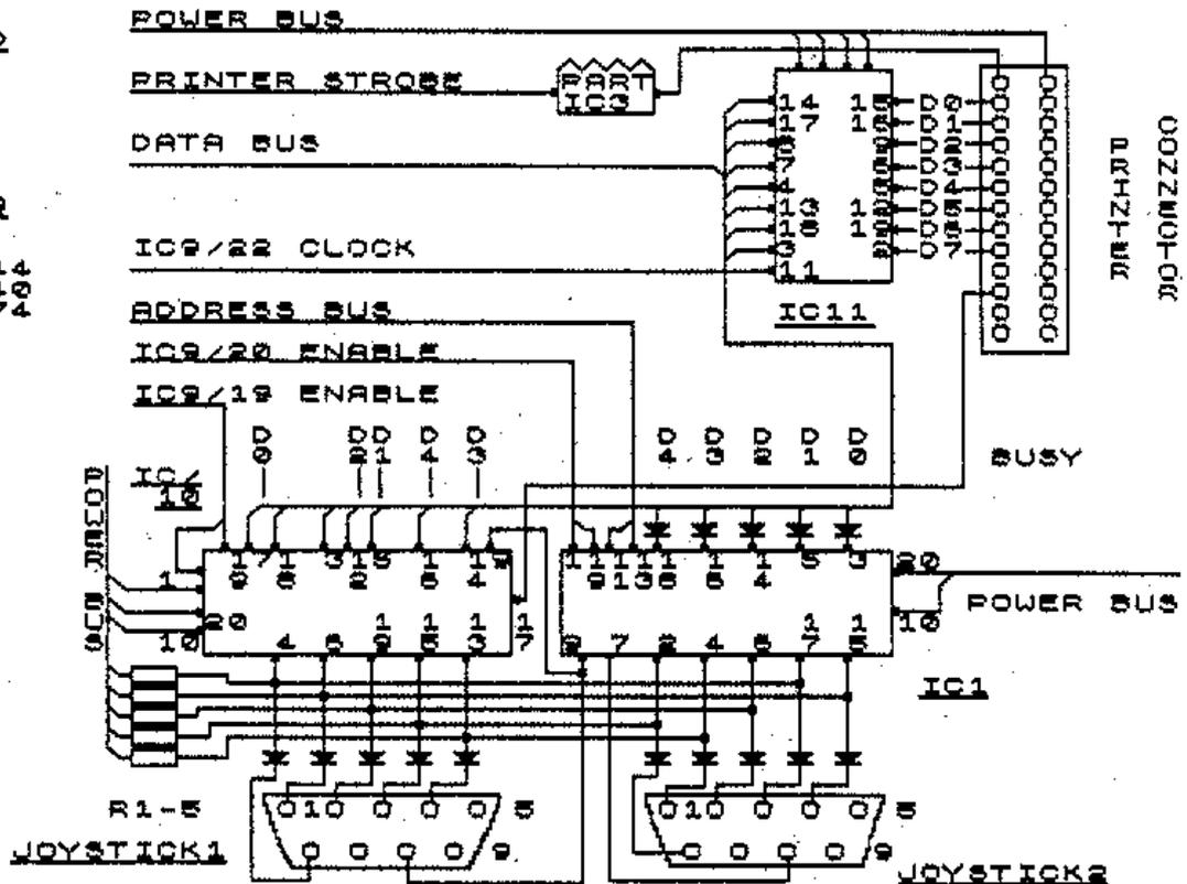
maximum length of the printer cable is 2 meters. Any greater and a problem known as 'skew' arises. Skew is where data bits arrive at the printer at different times. Some simple tests on my interface shows that the full alphabet can be sent to the printer in about 10 milliseconds (1/100 sec). This equates to a transfer rate of about 2,600 characters per second. The fact that most printers print 150 characters or less per second proves the need for the BUSY line.
