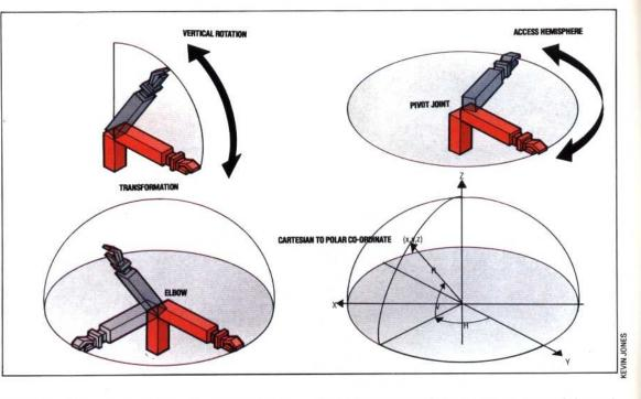
another distance variable, z). So by using cylindrical co-ordinates it would be very easy to develop a system that could pick out any object from a specified position inside the can.
