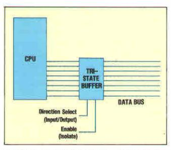
Eight such tri-state devices are combined into a single integrated circuit. The diagram above shows how this integrated circuit links the data bus with the CPU. The diagram also shows the 'enable' and 'direction select' lines, which put the eight tri-states into the required operative state. Such circuits can also be used for connecting other devices, such as input/output peripherals, to the data bus.
