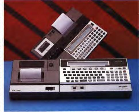
programs. As an additional option, the command PASS allows programs to be protected with a password. Line numbers in the PC-1251's BASIC are limited to the range 1 to 999. When in the mode for entering programs, two cursor keys allow the programmer to scroll up and down over the program lines. A further two cursors allow
