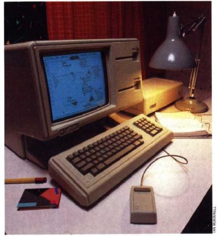
resolution of  $720 \times 364$  pixels. This permits a variety of different typefaces for text, as well as the kind of graphics shown in this feature. The Lisa's design incorporates special chips and circuitry solely dedicated to drive this display and rapidly move the images.
