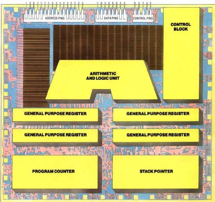
The computer's function is controlled by the CPU – the Central Processing Unit. The words can be interpreted fairly literally: Central – at the heart of the computer; Processing – it does the work; Unit – it stands alone. A very simple computer (see illustration) could consist of nothing more than a CPU, some memory and some I/O (input/output) circuitry.
