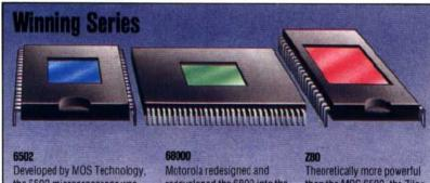
the 5502 microprocessor was to become, with Zilog's Z80, the mainstay of the microcomputer industry. It utilises a 16-bit address bus and an eight-bit data bus. Chief amongst its peculiarities is the organisation of its registers. There is only one accumulator, but the whole of memory page 0 can be used as general-purpose registers
