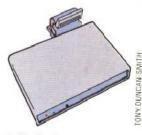
For The Spectrum The VTX 5000 is a modem specially designed for the Spectrum and has all the software you need built-in. It sits under the Spectrum and connects to its expansion connector
