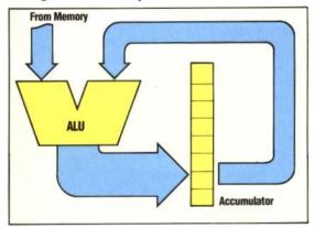
The numbers in the accumulator and memory have an eight-bit word length. The bits that make up the numbers travel through the ALU in parallel and the operation is carried out on all eight bits simultaneously. In order to describe the circuitry of the ALU, let us take just one of the eight bits and design a circuit that will allow us to carry out all six of the different functions. We shall call the bit from the first operand A and that from the second operand B.
