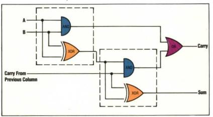
By adding on small circuits to the full adder it is possible to show how the adder's gates can be adapted to perform the other functions of the ALU. We shall set up a series of control signals to do this, the first of which is known as the *mode select* signal. The 'carry from previous column' input is used during arithmetic operations but is not required during logical operations. The mode select signal switches the carry input on or off. This is easily achieved by using an AND gate.
