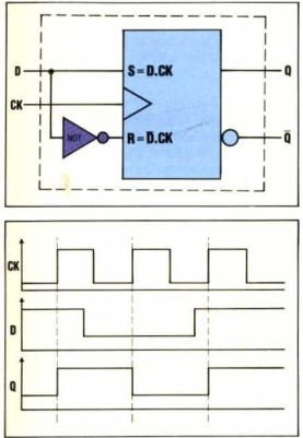
It can be seen from these graphs that the output Q can only change during a LO to HI transition of the clock. Consequently, the D-type is called a 'leading edge triggered' flip-flop.
