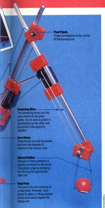
maintain the servos in their current position. These numbers may be altered by the user, and while the system is in Edit mode the servo motor being adjusted will move as changes are made, allowing the arm to be positioned to the user's satisfaction. Once the operator is happy with the positions of each of the motors, Return must be pressed, whereupon a new Robol line is displayed and the next series of movements can be programmed.
