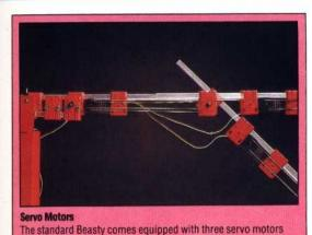
connected to an interface box. Servo motors are popular motors
