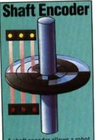
A shaft encoder allows a robot to know how far it has moved by measuring how much the axles of its wheels have rotated. The device is a calibrated disc, which is fitted on a shaft or axle. The circular plate is divided into a number of concentric rings, each marked out in areas that are either transparent or opaque. With a light source and a light sensor for each ring it is possible to work out the exact orientation of the shaft.
