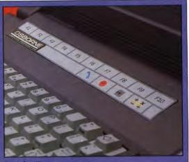
Above the main keyboard is a touch pad — similar to the keyboard used on the Spectrum and ZX81 — that contains the 10 programmable function keys. Below the function keys are the icons that are used to call the Encore's BOM based programs.
