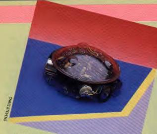
NAME: Memocon Crawler TYPE: Floor Robot PROGRAMMABLE: Yes SOFTWARE PROVIDED: NO SENSORY FEEDBACK: NO PRICE: £34.99
