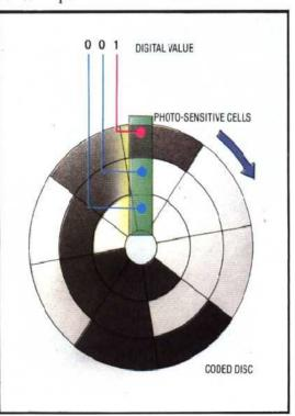
arrangements, radial patterns are also used to encode angular movement, such as that of a joint in a robot arm.
