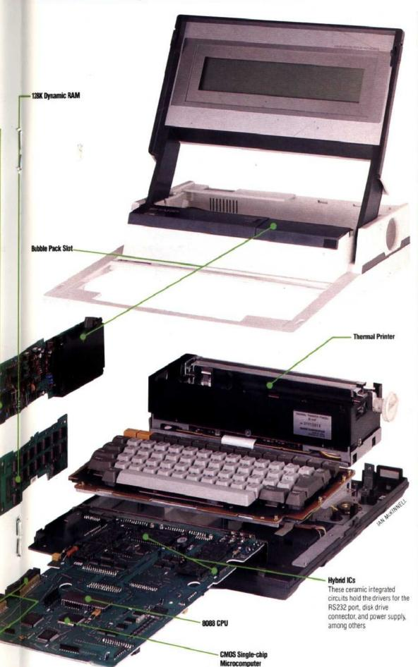
This chip controls the operation of the entire system, and shuts down the 8088, I/O chips, etc. when they are not being used, to
