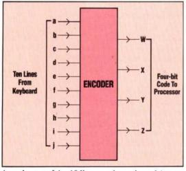
As only one of the 10 lines can be activated (or *set high*) at any one time, the truth table for the encoder will be:
