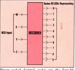
Binary-coded decimal codes are the four-bit binary representations of the decimal digits 0 to 9, and therefore the decoder will have four input lines. As any combination of the four lines can be set high, there are 16 possible inputs. We are only interested in the first 10 of these combinations and
