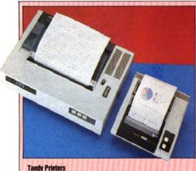
The Tandy Color Computer is well supported by a range of printers marketed by Tandy themselves. The CGP-220, for example, uses the ink-jet principle to produce seven colours, and is silent in operation. The cost is just under £500. At the other end of the scale, the CGP-115 at £150 uses four miniature ballpoint pens to produce colour printing and graph plotting
