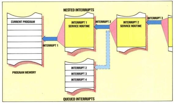
interrupts would be given priority and under no circumstances masked — thus giving rise to the concept of a *non-maskable* interrupt. Such an interrupt might come from a circuit that detects a drop in the mains supply voltage: its service routine would immediately start saving the current task while power remained.
