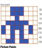
The user-defined characters representing the mine, the detector and the assistant are described. The pixel information is divided into eight bytes, with each byte being the binary 'picture' of one row of the shape
