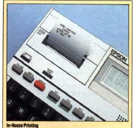
Small dot-matrix or type-roller printers have formed an integral part of cash registers — and even calculators — for quite some time, and Epson, who started life as printer manufacturers, were quick to incorporate the idea into their HX-20 portable. This dot-matrix printer is capable of graphics as well as character output
