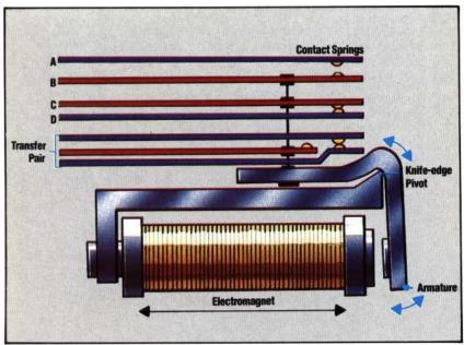
The relay makes and breaks contacts under the action of small movements in the armature. An appropriate voltage applied to the solenoid coil generates a magnetic field that attracts the armature. As the armature swings in towards the coil the spring contacts attached to the other end of the armature are made to move vertically upwards.
