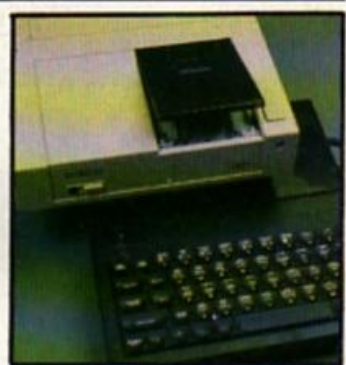
Radofin's 2.8-inch disc drive
