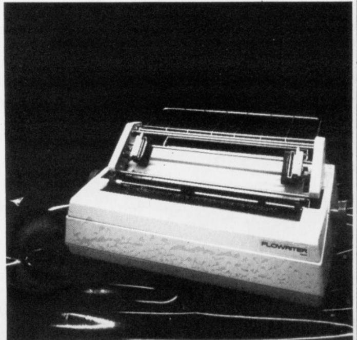
By offering the extra intelligence – it has its own Intel 8085 microprocessor and 8.5K bytes of RAM memory on board – the *Flowriter* takes the burden off your computer; the result is much faster throughput.
