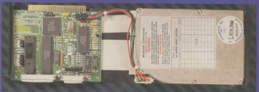
**2** This is a hard card, but it shows all the elements of a hard disk in one neat package. The disk drive itself can be seen to the right. This is completely sealed in so you'll just have to take our word for it that there is a disk in there. The disk is linked via a strip of ribbon cable to the controller circuitry. On a conventional hard disk, the disk drive and the controller circuitry are mounted in separate parts of the computer – the hard card keeps them in one place.
