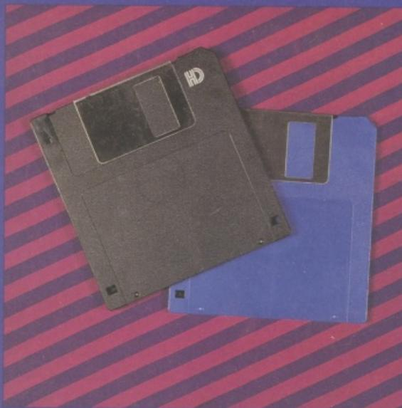
Taking over from the 5.25-inch floppy disk is the increasingly popular 3.5-inch disk. It is smaller and more resilient than its predecessor. 3.5-inch disks come with either 720K or 1.44 Mb of capacity (the one labelled HD in our picture is one of the larger capacity disks). Astute Amiga, ST or Mac owners may notice that these look the same as their floppy disks. This is because they are the same.
