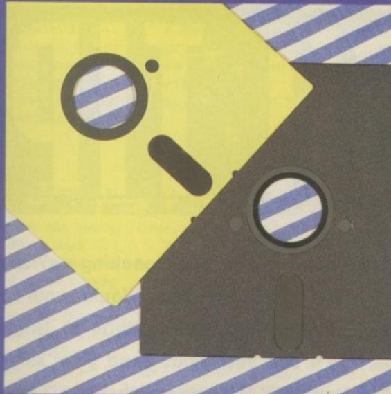
**1** The first PC floppy disks were 5.35-inch disks holding 160K. The current standard is still the 5.25-inch disk, but these can now hold 360K (the 'double density' disks) or a massive 1.2 Mb (so-called 'high density disks'). From high-street retailers, floppies are comparatively expensive – buying a minimum of ten at a time from a mail-order outlet can save pounds.
