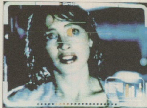
• This picture is a composite image created using a genlock. It combines a video image (the girl) with Amiga graphics.
