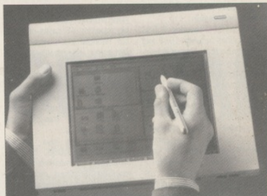
• The 3125 also offers the first commercial implementation of a pen-based Windows 3. Microsoft is known to be keen to further distance itself from the IBM platform so when Big Blue eventually gets round to releasing its own pen-input machine in 1992 or 1993 don't expect to see a version of Windows running on it.
