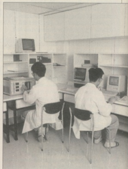
• Quality control testing of diskettes. To ensure the entire surface is error free, the area between the tracks and the area between the tracks are tested.
