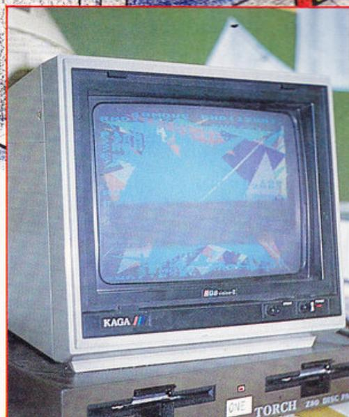
This is what the image looks like on an RGB monitor. You should be able to see, by comparing it to the same image on an ordinary TV in the picture opposite, that the resolution and quality of the RGB picture is much higher than that of the television screen.
