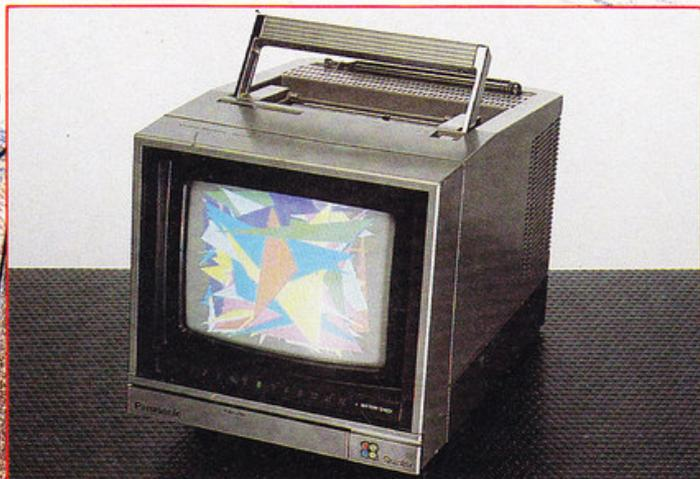
At the top of this page, you'll see what the display from a BBC Model B looks like on an ordinary TV set. The BBC has the capacity to run all three of the chief sorts of monitors; RGB, composite video and UHF TV so we have picked it to display the same picture on two screens. The first of those screens is at the top of the page, while the second is at the bottom of the opposite page.
