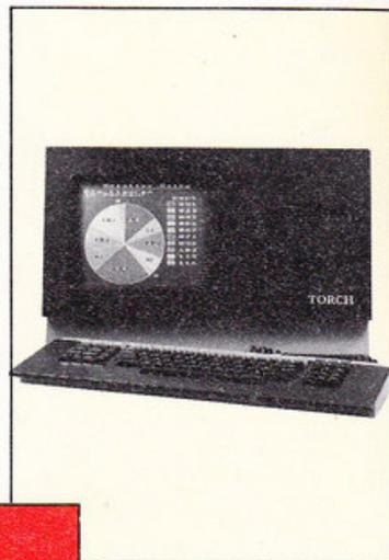
A variety of monitors are popular with certain computers. On Torch computers (top photo), a colour monitor is built into the machine and you don't really have a choice (although the machine does allow for hooking up more than one monitor at a time). Some monitors, such as the early Cabels (see photo opposite), had controls for things like vertical and
