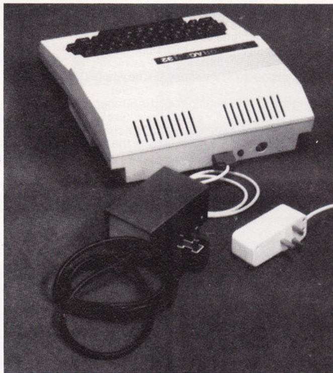
You could use a special protector, like The Plug (left) or stick with the Dragon's built-in regulator (right) to keep your power supply clean.
