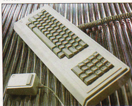
Lisa's keyboard looks ordinary but it's different: every key may be programmed individually.
