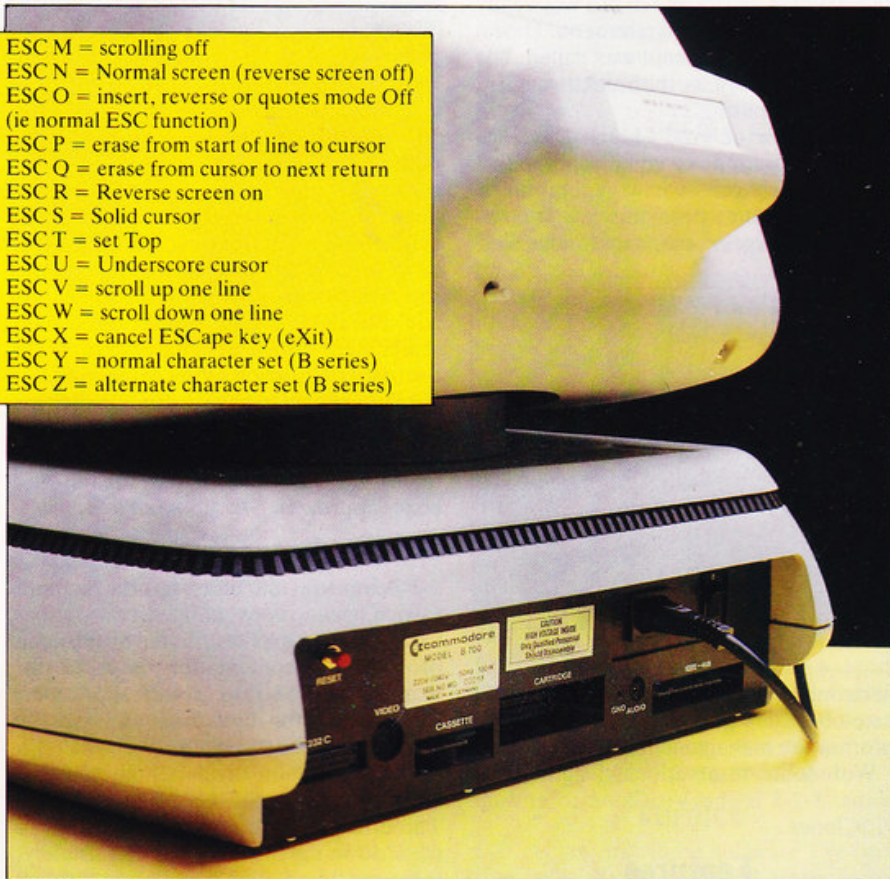
Reset button, RS232, video, cassette (would you believe!), cartridge, Earth, audio and IEEE 488 — connections in that order.
