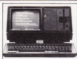
The Winchester-equipped dual processor Cifer Club micro.
