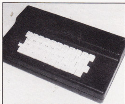
Fuller's ZX keyboard adapted by TEC with extra switches.
