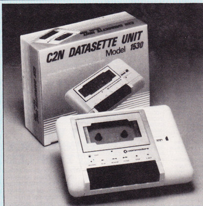
COMMODORE CASSED — Commodore decided it was about time it re-vamped its ugly cassette unit. The result is the new C2N 'datasette' pictured. Apart from the new casing there are few changes from the current version. The tape-heads have been improved to withstand oxide build-up and the electronics have been tweaked to make the machine more reliable. It costs £46.
