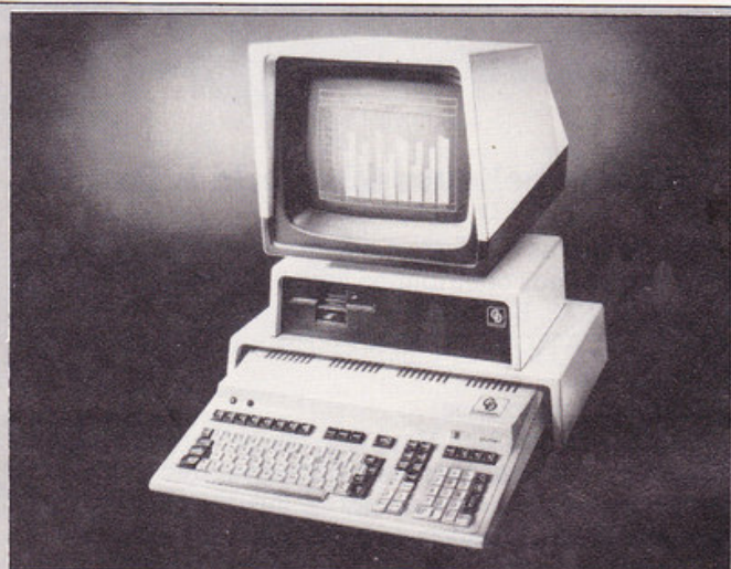
FLOWER POWER — This latest IBM PC imitator should reach our shores by June. Called Tulip System 1, it is produced appropriately enough in the Netherlands by Computdata and should sell here for £3,700. The 16-bit micro, based on the 8086 microprocessor with a clockspeed of 8Mhz, has 128K of RAM expandable to 896K. It runs MS/DOS and CP/M-86 and has a floppy disk capacity of 750K along with 5 or 10Mb hard disks. As far as graphics go, it has low resolution as standard with high resolution as an option.
